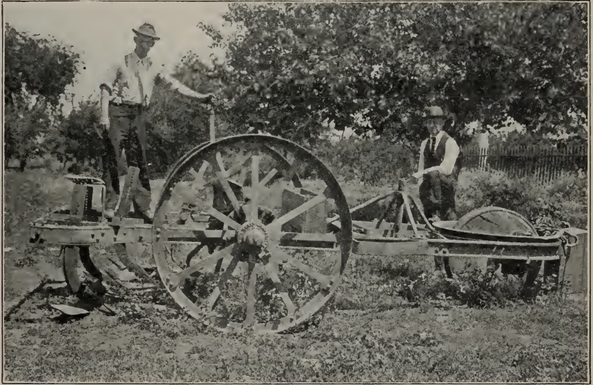
Fig. 9.—A very efficient type of weeder and sub-soiler, drawn by 80 h.p. Holt tractor and running 16 to 18 inches deep. With this machine it is possible to grow sugar beets without hindrance from morning glory. The implement is made at Liverpool, England.
